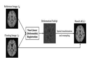
Image registration is a crucial and fundamental procedure in medical image analysis. The aim of registration algorithm is to obtain a spatial transformation that can align a floating image to a reference image. The resulting anatomical correspondences allow image comparison for applications such as population analyses, longitudinal studies, and image-guided interventions.
