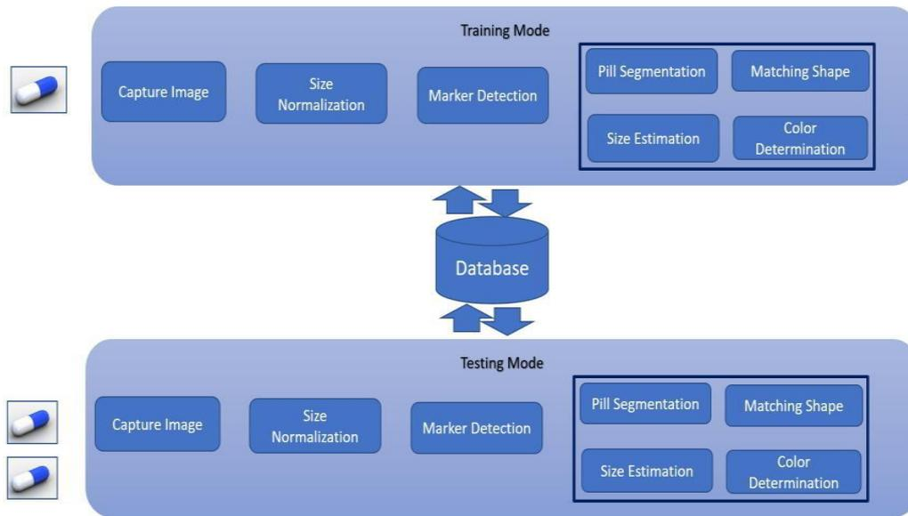
There are two different ways that our drug pill detecting system can function. In the first mode, an image containing the marker and pill is first taken in order to create and store pill profiles. The process of obtaining an image from a source and resizing it to a standard size is known as image acquisition. When the marker is detected, the system analyzes the pill's size, shape, and color to identify it and stores all relevant data in its database for later retrieval.
