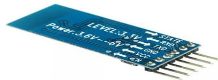
**Fig.2: Serial Bluetooth Transceiver**
