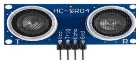
**Fig.3: Ultrasonic sensor HC-SR04**
