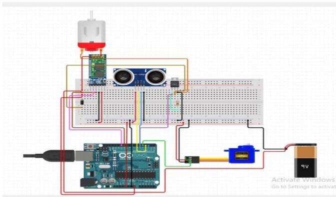
**Fig. 8: Circuit Diagram-Smart Autonomous Floor Cleaning Robot**
