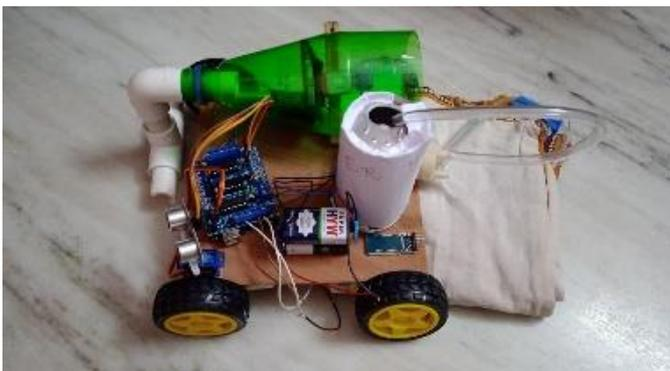
**Fig. 9: Prototype of autonomous floor cleaning device**
