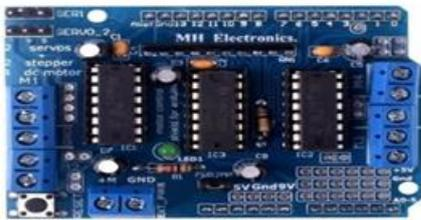
Fig. 5: L239D DC Motor Drive Shield
