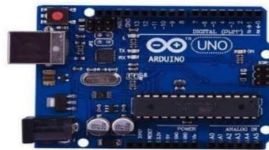
**Fig. 1: Arduino UNO R3 ATmega328P Microcontroller**
