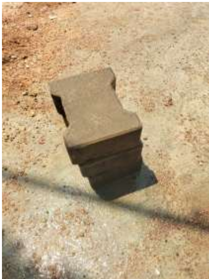
Fig. 1. I-shaped paver block specimen ( 200 \times 160 \times 60 mm) used in the present study.
