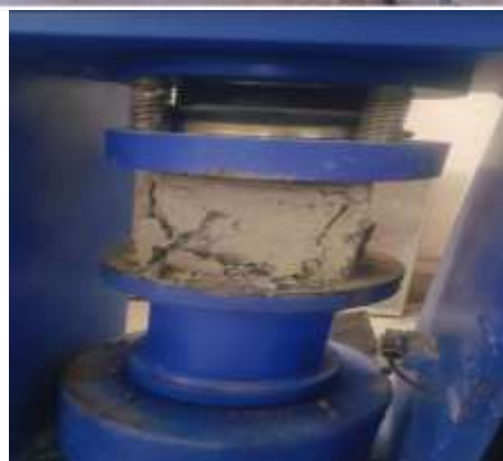
Fig.3.9: Testing machine for compressive strength at GIFT
