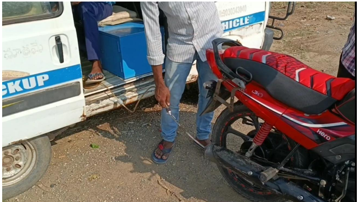
Figure 6.4 P.U.C Test on Vehicle
