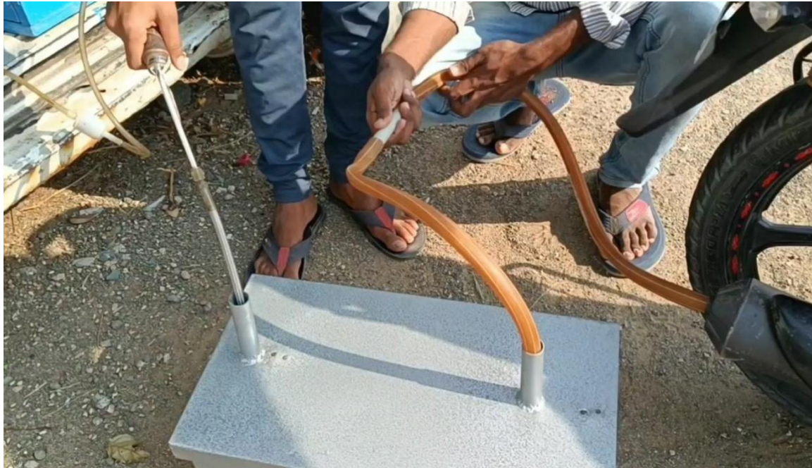
Figure 6.5 P.U.C Test on Vehicle with Aqua Silencer Setup & Normal Water
