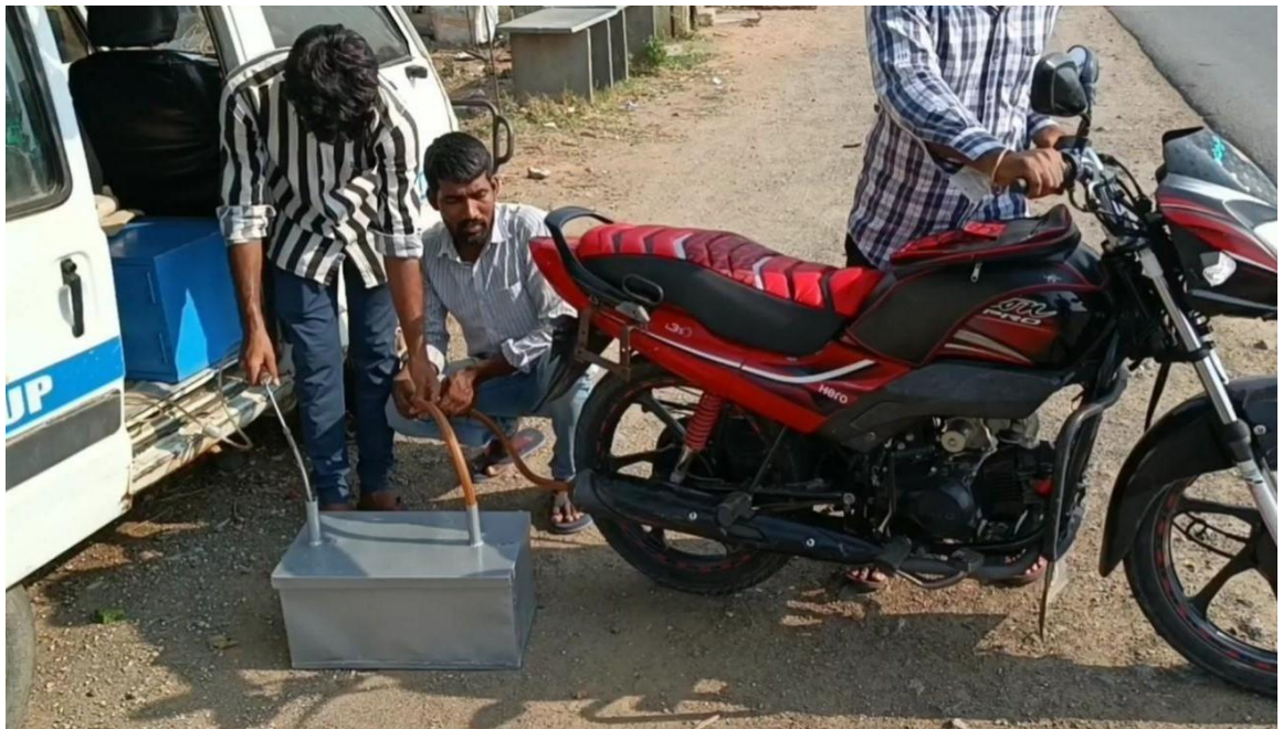
Figure 6.7 P.U.C Test on vehicle with Aqua Silencer Setup and Green Algae Water
