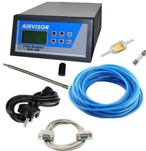
Figure 6.2 P.U.C Machine Airvisor Setup (Gas Analyser)
