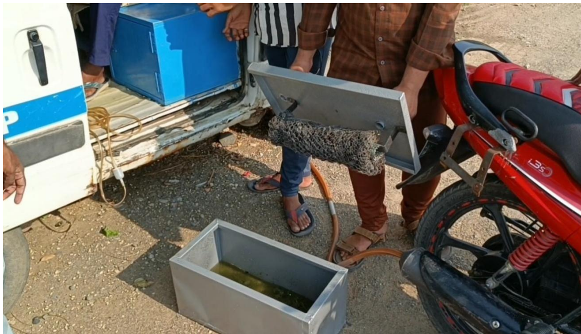
Figure 6.6 Aqua Silencer Setup with Green Algae Water
