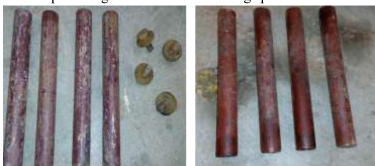
Fig 1.1 Micro-piles of 16 mm and 20 mm diameters with nut and bolt system
