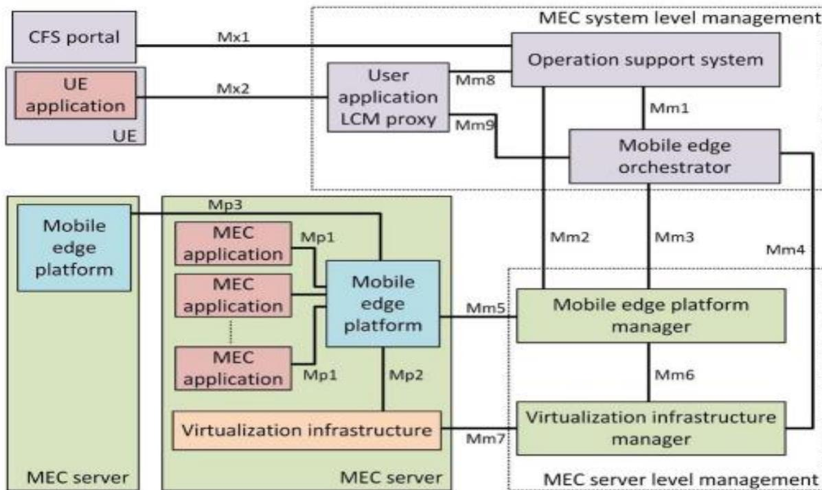
Figure 3: Mobile edge computing reference architecture [8]
