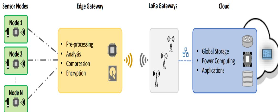
Figure 4: Architecture with integration of Edge Computing [7]
