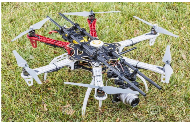
Figure 6: UAV with camera and GPS for Automatic Verification
