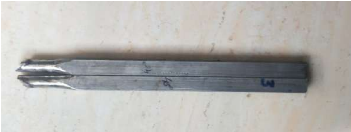
Figure 3.6 Tensile testing of welded specimen (0°, 15°, 30°, and 45°)
