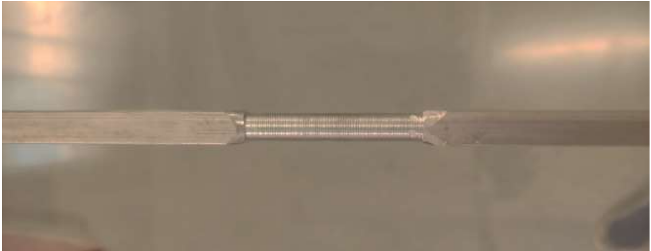
Figure 3.3 Surface Finishing before TIG welding
