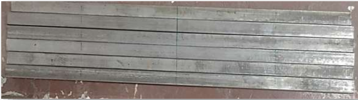
Figure 3.1 Raw mild steel rods used for specimen preparation
