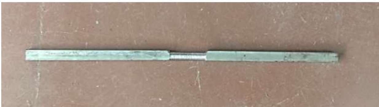
Figure 3.2 Machining of mild steel rod for specimen preparation
