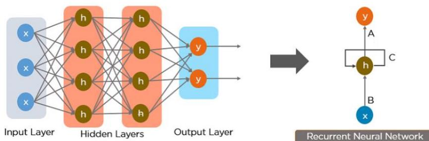
Fig 8.2. Simple Recurrent Neural Networks (RNNs) Model
