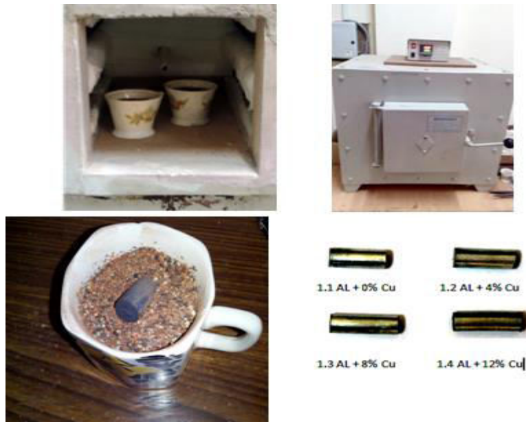
Figure 4.4: Chronological order of sintering arrangements
