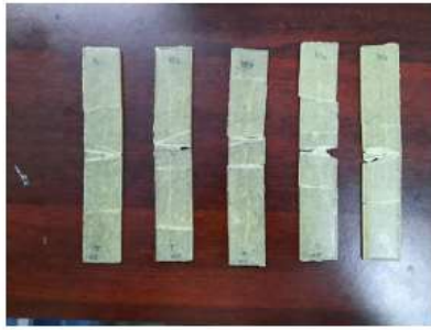
Figure 10 Epoxy Samples with milled Kevlar fibers after testing
