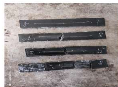
Figure 9 Epoxy Samples with milled Carbon fibers after testing
