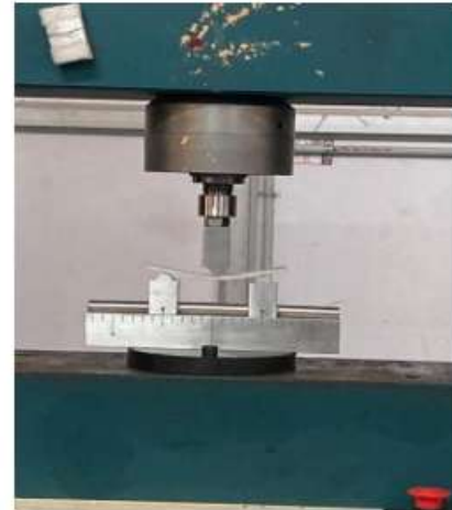
Figure 11 Three-point flexural test
