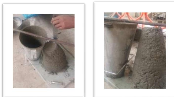
Figure No. 5 Workability of the fresh concrete (slump test)
