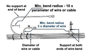
• Different cables used in avionics, including their bend radius and potential impact: Table 2 represents all the different cable types used in avionics and its maximum allowed bend radius
