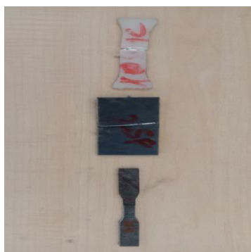
Fig 6: Specimen for testing according to ASTM STD
