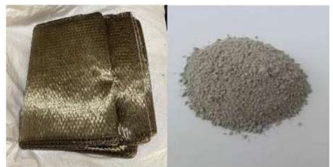
Figure 2: Basalt Uni-Directional Fibre (left), Powdered Basalt Filler (right)
