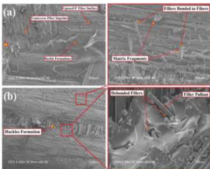
Figure 44: SEM Micrographs of fractured surfaces after flexural testing of (a) baseline basalt/epoxy samples (b) 1% wt. basalt filler modified basalt/epoxy samples. To the right, two insets of (b) showing close-up of the marked regions.
