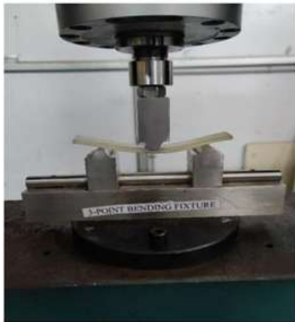
Figure 14: Three-Point Flexural Test
