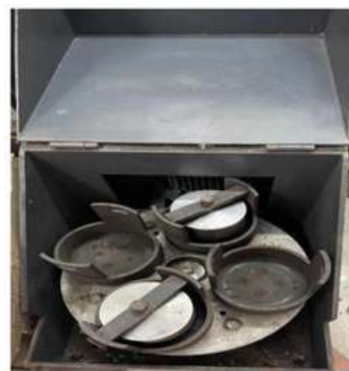
Figure 5: Planetary Ball Mill Setup
