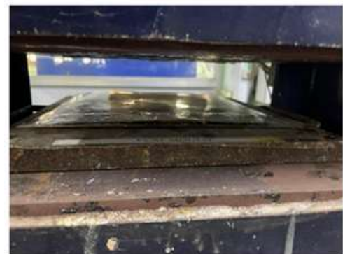
Figure 30: Compression Moulding in the Moulding Chamber
