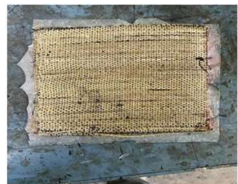
Figure 31: Areca Nut/Epoxy Sample Post Compression Moulding
