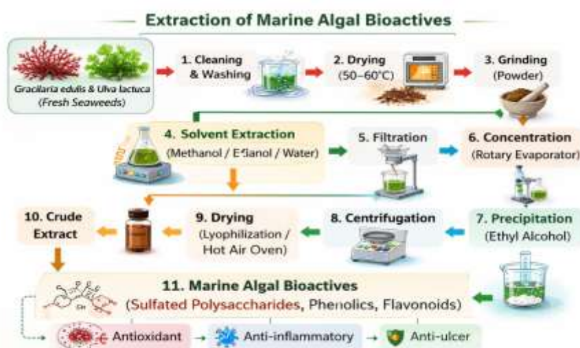
Figure 5. Schematic representation of the extraction process of marine algal bioactive from Gracilaria edulis and Ulva lactuca .
