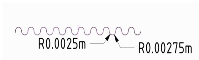
Fig.2. Corrugated Model (Side view)
