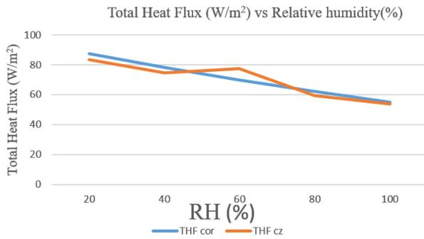
Fig.7. At 18°C, THF at different RH
