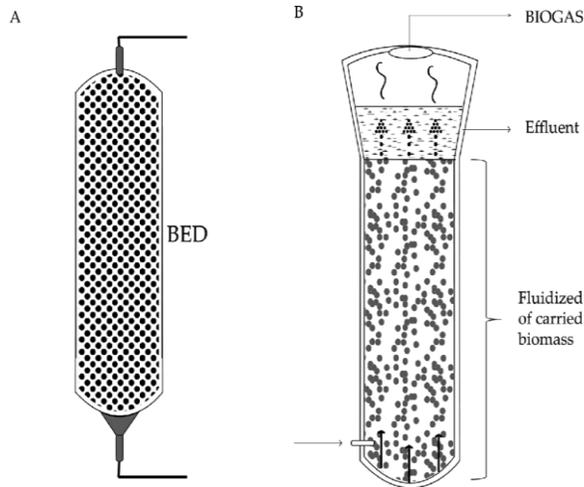
Figure 1 – Schematic of fluidized bed
