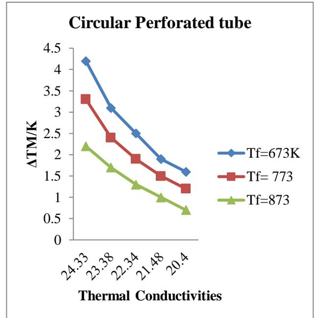
**Figure 7** Temperature distribution and thermal conductivities in CFB boiler tube with circular shaped inclined perforations.
