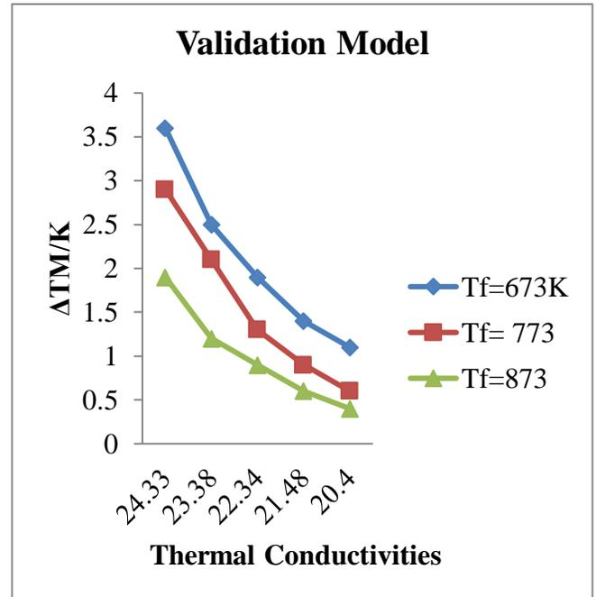
**Figure 3** Temperature distribution and thermal conductivities in CFB boiler tube with fin (Validation model).
