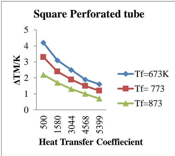
**Figure 4** Temperature distribution and heat transfer coefficients in CFB boiler tube with square shaped inclined perforations.
