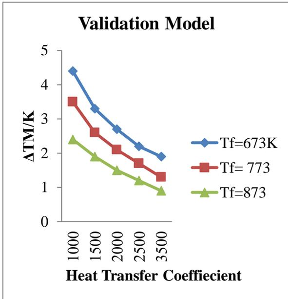
**Figure 2** Temperature distribution and heat transfer coefficient in CFB boiler tube with fin (Validation model).
