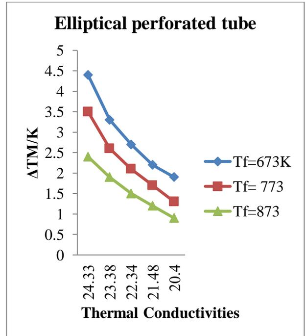
**Figure 9** Temperature distribution and thermal conductivities in CFB boiler tube with elliptical shaped inclined perforations.
