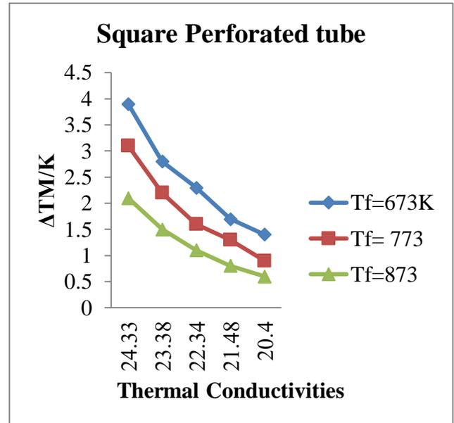
**Figure 5** Temperature distribution and thermal conductivities in CFB boiler tube with square shaped inclined perforations.
