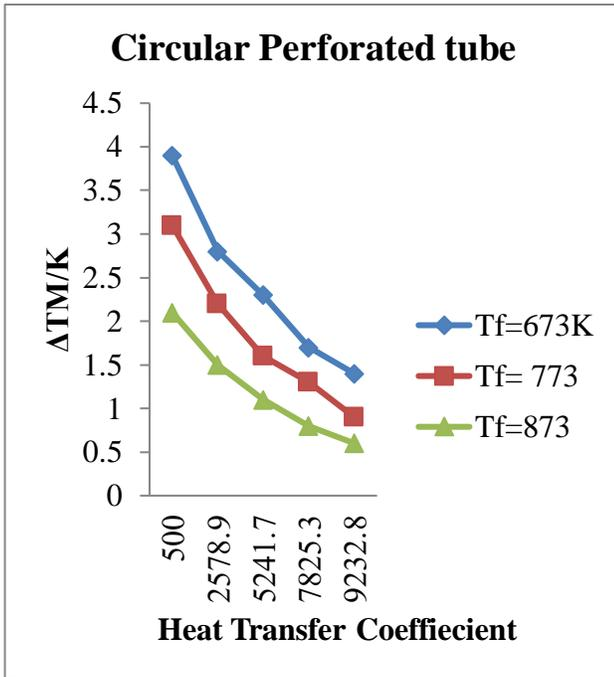
**Figure 6** Temperature distribution and heat transfer coefficients in CFB boiler tube with circular shaped inclined perforations.
