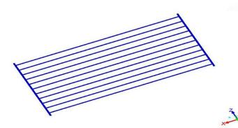
Figure 5 - Harp absorber meshed
