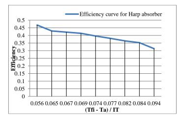
$\begin{array}{l} Figure \; 11-Plot \; of \; Efficiency \; v/s \; [(T_{fi}-T_a) \; / \; I_T] \; for \; F_R \\ of \; Harp \; system \end{array}$
