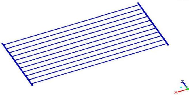
Figure 5 - Harp absorber meshed
