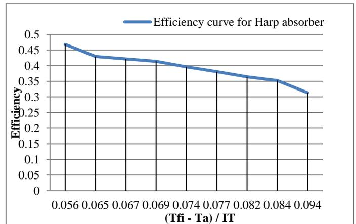
Figure 11 – Plot of Efficiency v/s  $[(T_{fi} - T_a) / I_T]$  for  $F_R$  of Harp system
