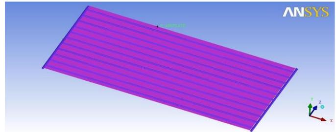
Figure 4 – Harp absorber with plate
