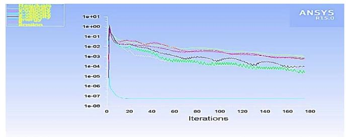
Figure 9 – Residual plot of Harp absorber
