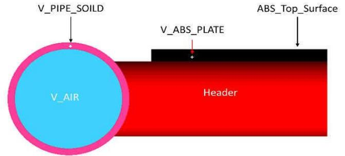
Figure 3 – Zones in the geometry
