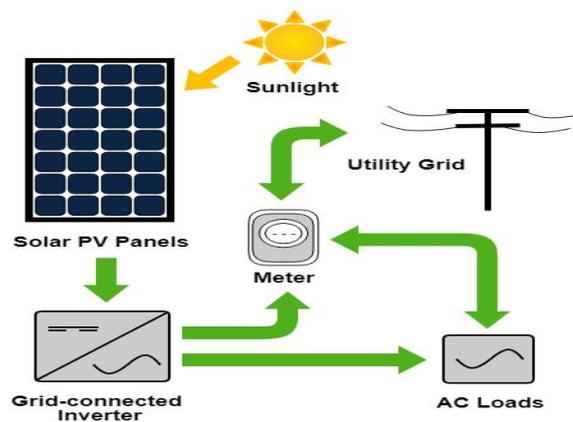
Fig.1. Simplified Grid connected PV System
