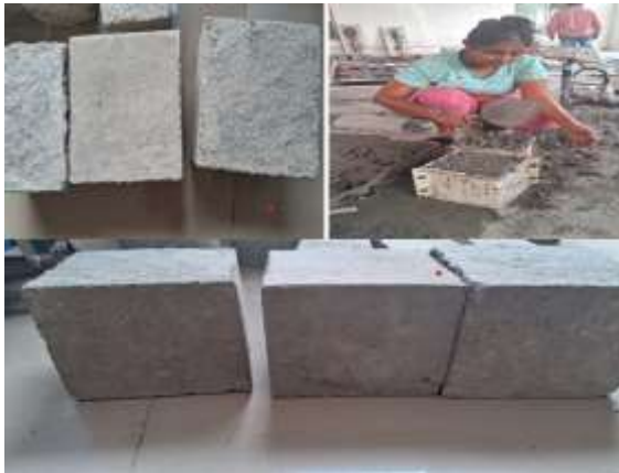
Fig 6: Casting process of compression strength of concrete
