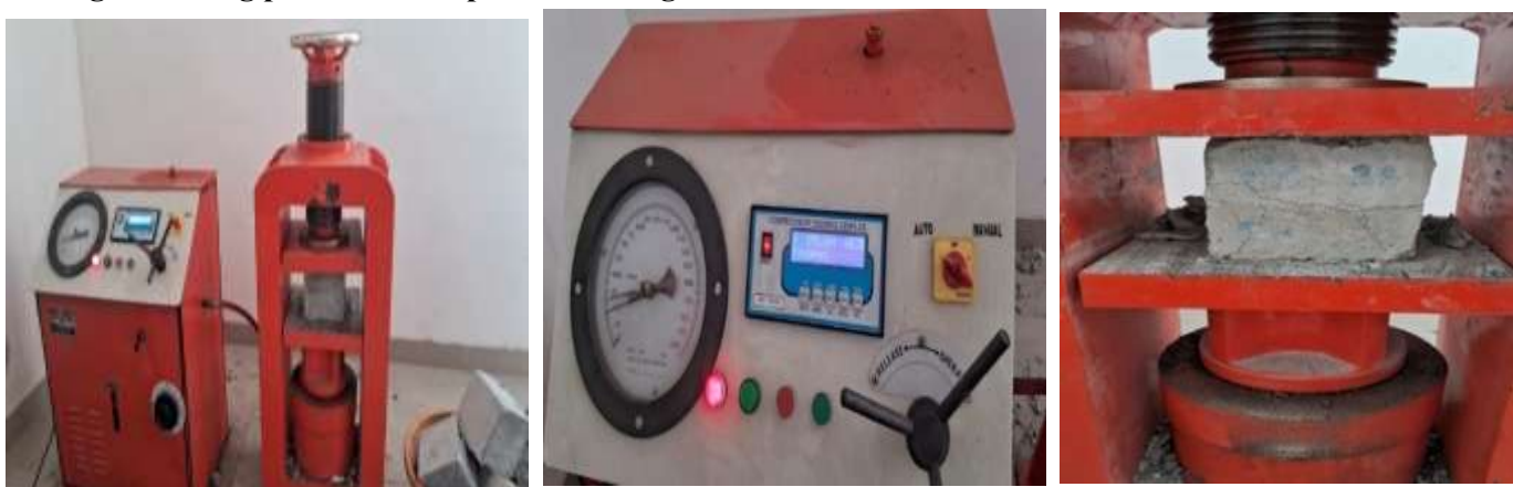
Figure 7: Test procedure of concrete compression strength.
