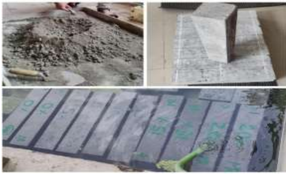
Fig 8: Procedure of casting of Flexural strength of concrete Table
