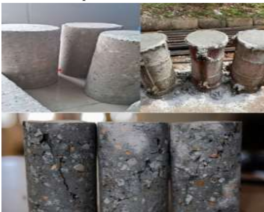
Figure 10: procedure of casting Split-Tensile strength of concrete
