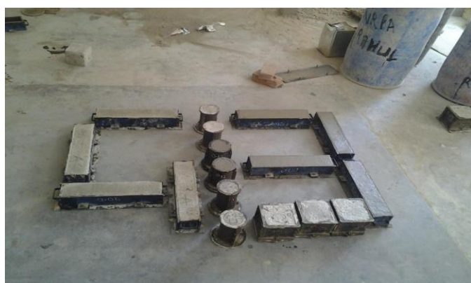
Fig-1: Concrete moulds filled with glass fiber
