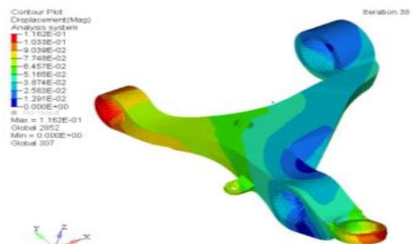
Fig.5.4 Displacement contour for the second load step at the last iteration.
