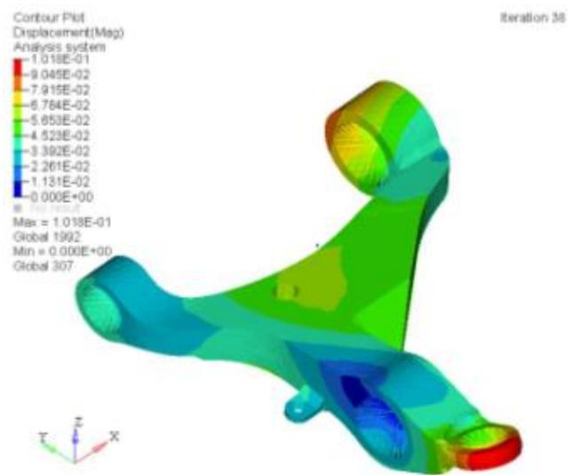
Fig.5.3 Displacement contour for the first load step at the last iteration.
