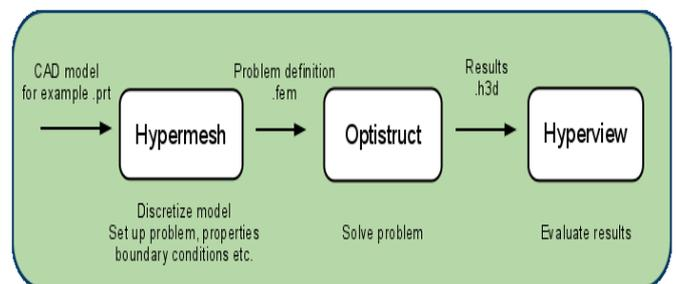
Fig.4.1 An overview of the workflow in Hyper works
