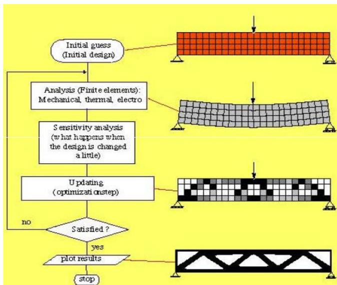
Fig.2.1 Flow chart of topology optimization process
