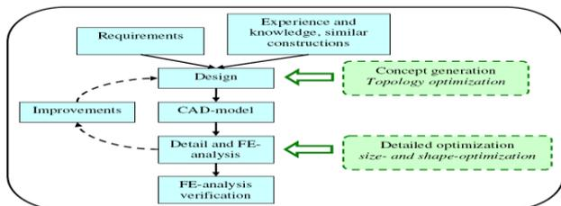
Fig. 3.1 Overview of the design process
