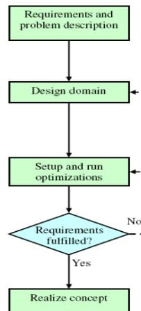
Fig.3.3 Concept generation process
