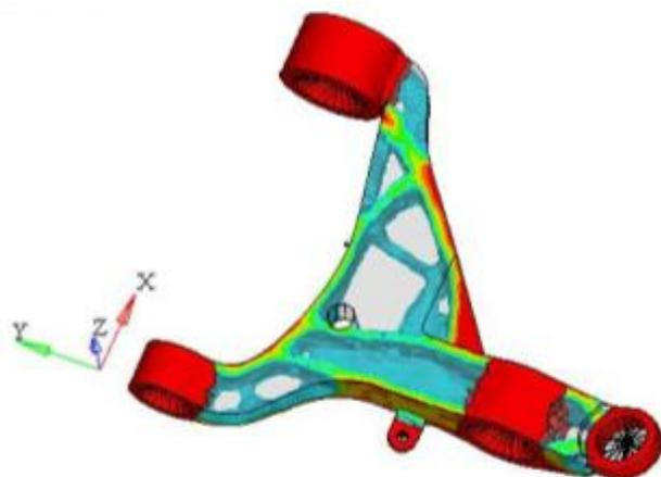
Fig.5.2 Iso surface plot of element densities.
