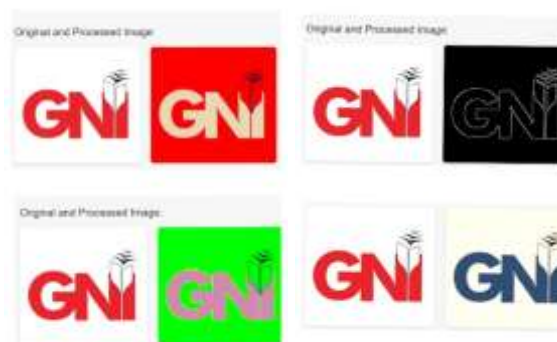
Figure 3: RGB images translated to different forms of images HSV (top left), Canny Edge (top right), HLS (bottom left), XYZ (bottom right) respectively by using Generative Adversarial Networks(GAN) for each format in different style.
