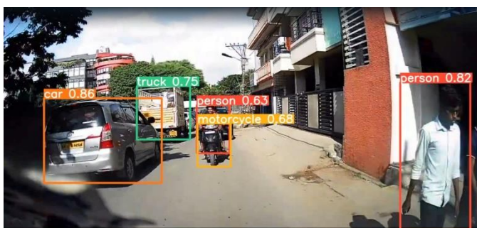
Figure – 4.1: Objects detected by YOLO model trained by COCO dataset.
