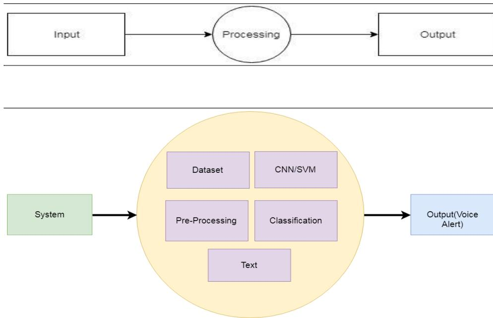
It consists of input which is given by the camera module then it is passed to the processing block in which the input is first pre-processed and then recognized and classified into specific traffic signs it is corresponding to with the help of a trained dataset and CNN algorithm. After this, the output is generated and displayed on the monitor.
