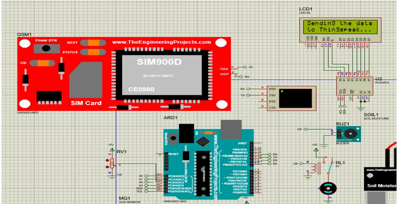
Figure 48: Proteus Simulation of LCD, NODEMCU ESP8266 Module with Arduino
