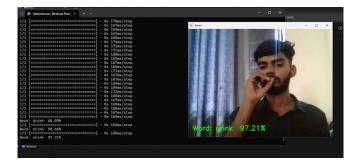
Realtime testing involved capturing ASL gestures using a camera and processing the frames through the trained model. The system performed well in controlled environments with proper lighting and minimal background interference. However, performance decreased in dynamic environments with varying lighting conditions, hand occlusions, and complex backgrounds.
