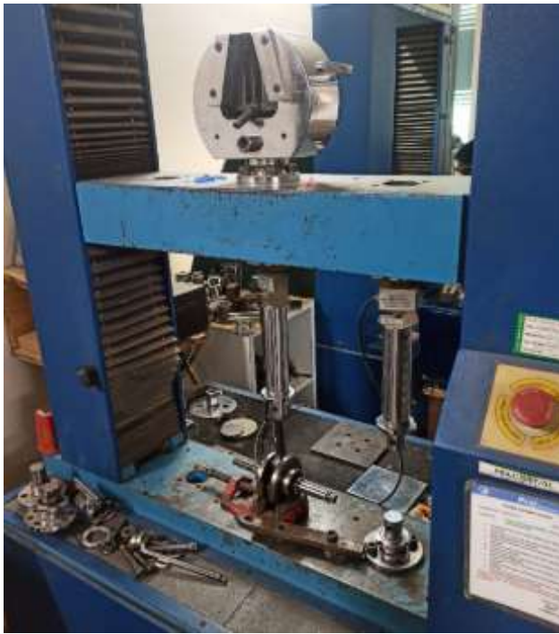
Fig-41: Specimen under compression test using a UTM.
