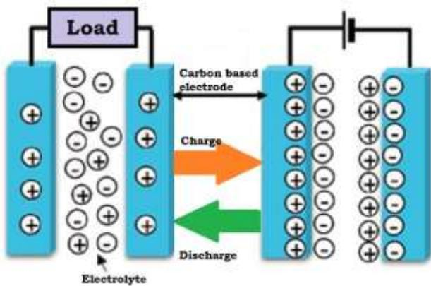
Fig.1 ultracapacitor working
