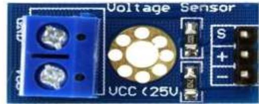
Fig.5. Voltage Sensor
