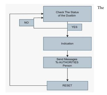
system uses an ultrasonic sensor to determine the amount of debris in the bin at regular intervals.
