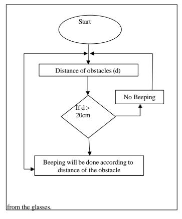
As stated in claim 1, as the visually impaired individual approaches an obstacle, the distance measured by the sensors relayed to the central unit will diminish. Consequently, the intervals between the buzzer's beeps will shorten, resulting in a faster beeping rate. Conversely, as the individual moves away from the obstacle, the intervals will lengthen, leading to a decrease in the frequency of the beeping.
