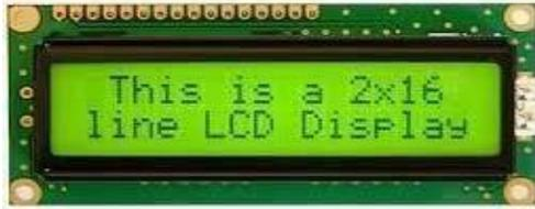
Fig-2: LCD Display
