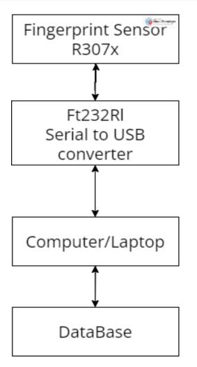
Figure 2. Block diagram of project's overall structure and components
