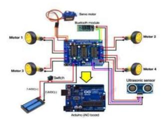
Fig.: Circuit diagram of voice controlled robotic car
