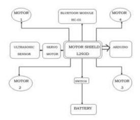
Fig.: Block Diagram of the model
