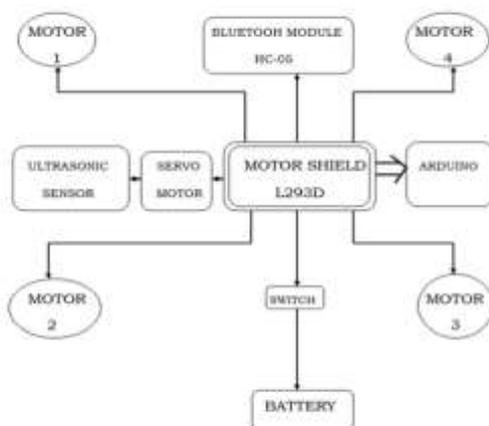
Fig.: Block Diagram of the model
