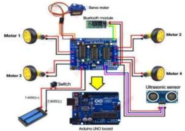
Fig.: Circuit diagram of voice controlled robotic car
