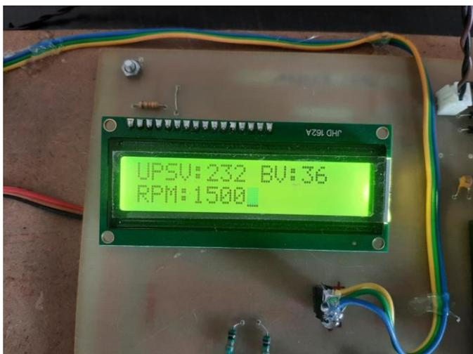
**Fig12.** Depicts the Voltage and RPM of the Colling Fan in LCD.
