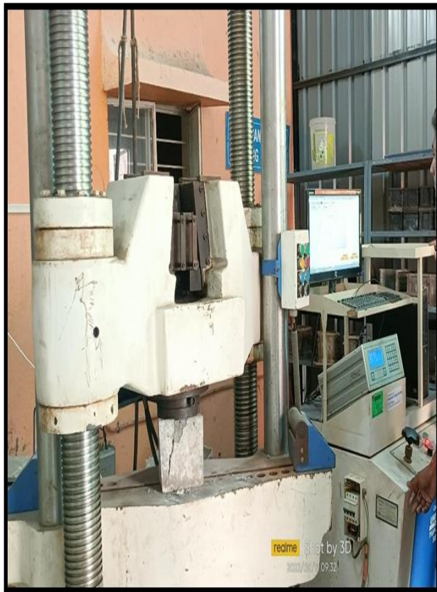
Fig No. 3.1 Compressive Test Carried Out on Universal Testing Machine
