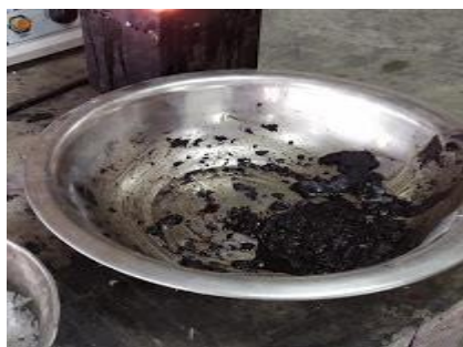
Fig.2: Sodium lignosulfonate mixed with kerosene
