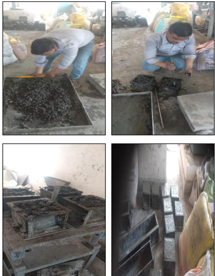
FIGURE 2. MIXING, MOULD FILLING. COMPACTING AND CUBES IN MOULD
