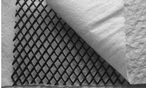
Figure 3. Knitted geotextile ,
