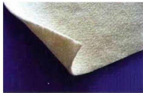
Figure 2. Non-woven geotextile,
