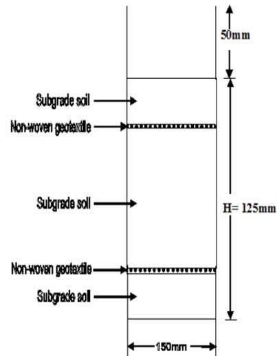
**Figure 1: Cross-sectional diagram showing the subgrade soil and non-woven geotextile layers**
