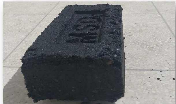
Fig No.: 2 Plastic Foundry sand Brick.
