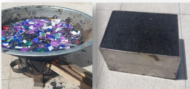
Fig No.: 1 Melting of plastic and moulding of brick.
