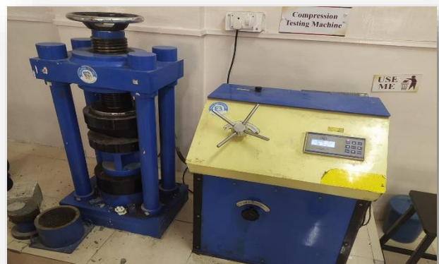
Fig No.: 4 Compressive Test of the Brick.
