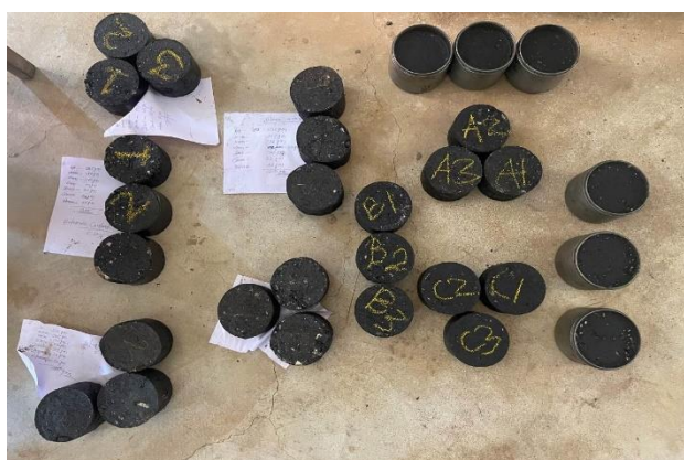
Figure Error! No text of specified style in document.3: Samples for Marshal stability and Flow test.
