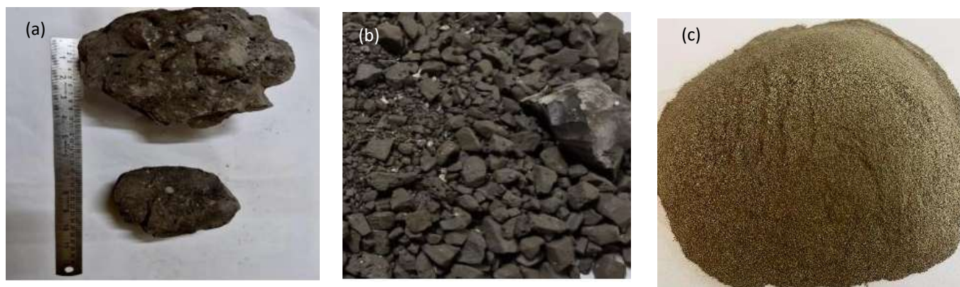
Fig.1 . Stages of BOF slag refinement: (a) raw slag stone, (b) crushed fragments, (c) ultra-fine
