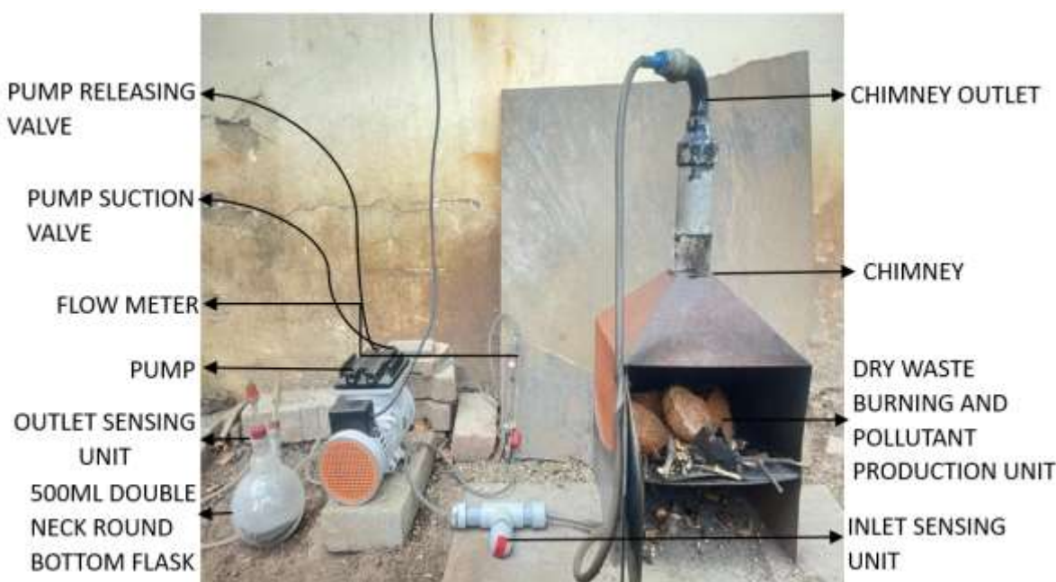
Fig.3 . Experimental setup for both Direct and Indirect Carbonation
