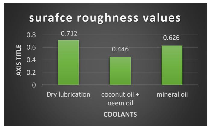
Figure 23 : Surface Roughness values with various coolants
