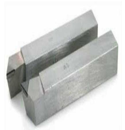
Figure 10: Single point cutting tool
