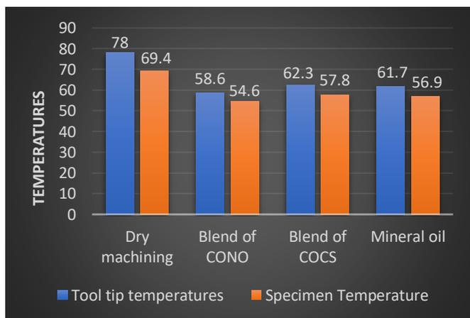
Figure 26: Recorded temperatures with various coolants
