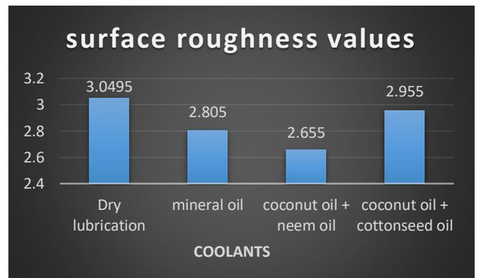
Figure 22: Surface Roughness values with various coolants
