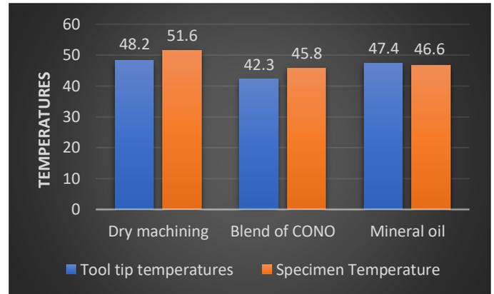
Figure 27: Recorded Temperatures with various coolants
