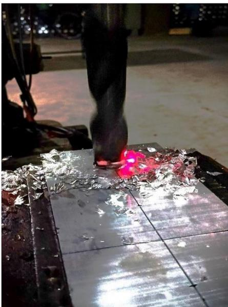
Figure 16: Drilling operation with 25mm drill bit on flat Al plate of 15 mm thickness
