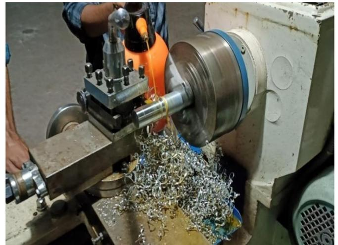
Figure 17: Turning operation with single point cutting on aluminium rod of 30mm diameter
